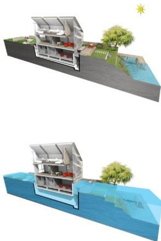
Figure 9.0: BACA Architects' Amphibious House – normal position (left) and flooded position (right)
