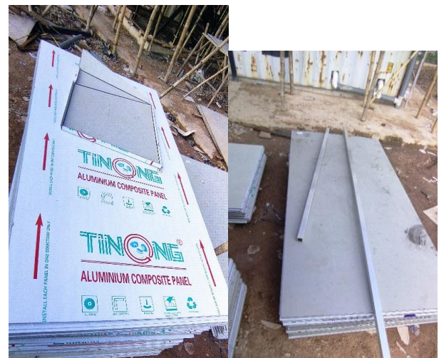
Fig 2.0: Image of Exterior cladding panels- Aluminum Composite panels for the Tech Hub at Helio Health and Tourism District, Enugu Source: Author, 2024
