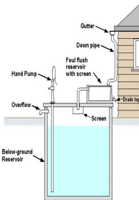
**Figure 1:** Diagrammatic representation of a harvesting system for rooftop rain-water
