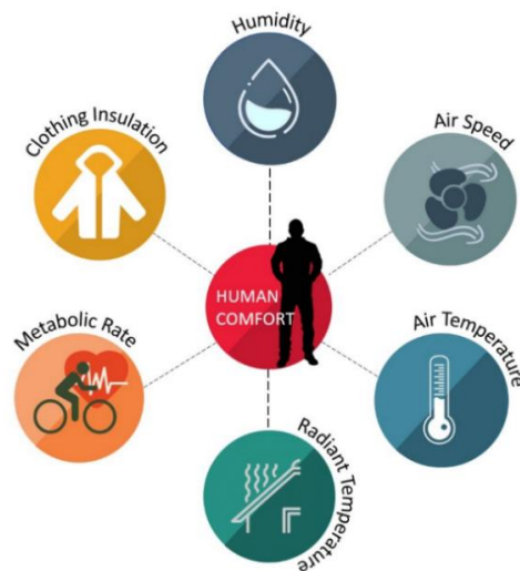
Figure 2: Environmental and Physical factors that influence human factors Source: Role of CFD in Evaluating Occupant Thermal Comfort, (2023).
